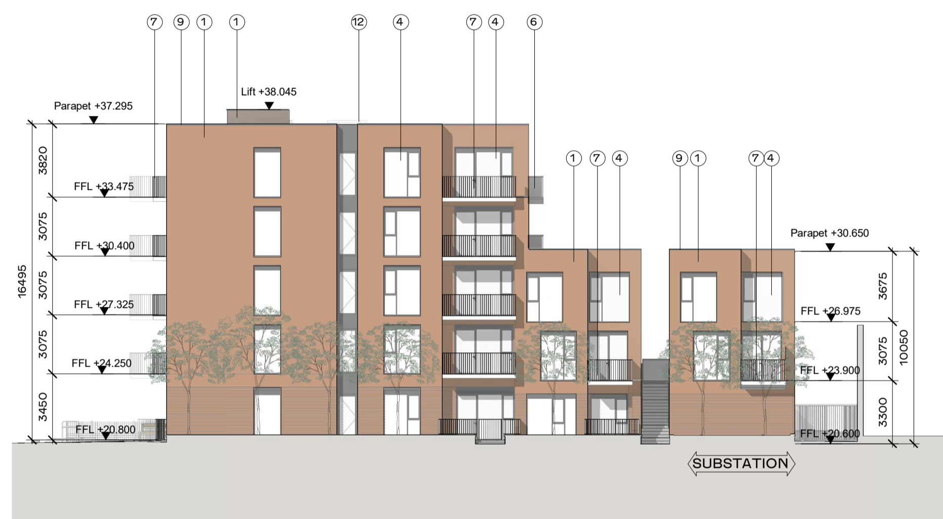
4 Block Elevation BG3 01 West Elevation 1 : 200
